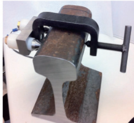
Original Modified Shunt Clamp (0 Ohms)
