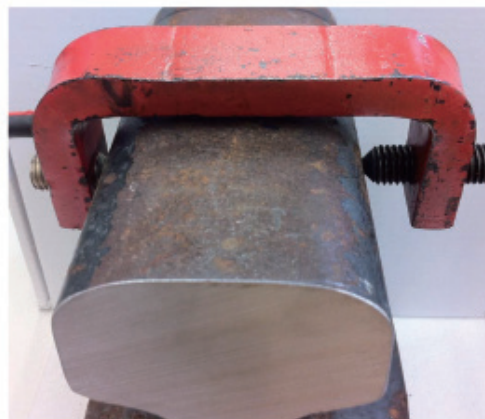
Rail Shunt Clamp (0.06 Ohms)
